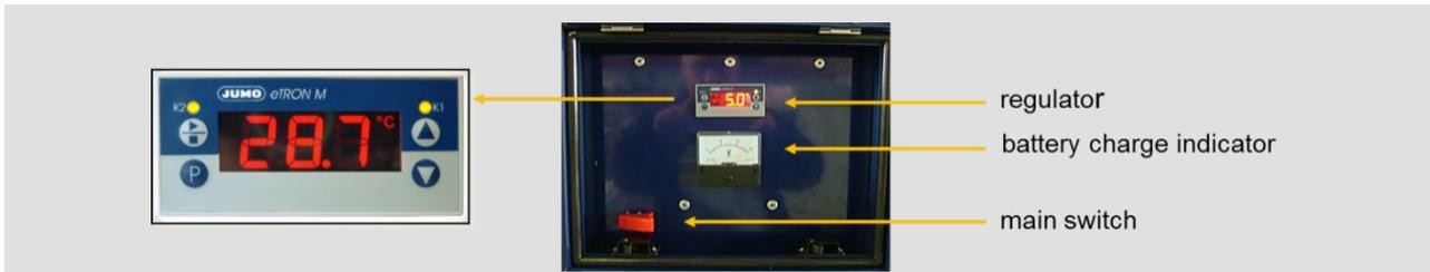
The customer selects the required temperature and the permanent air circulation provided by ventilators maintains a constant temperature in the cargo compartment.
