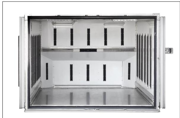
The cargo compartment has a loading height of 1,370 mm (53.9 in), providing space for 5 Euro pallets or 4 US pallets.
